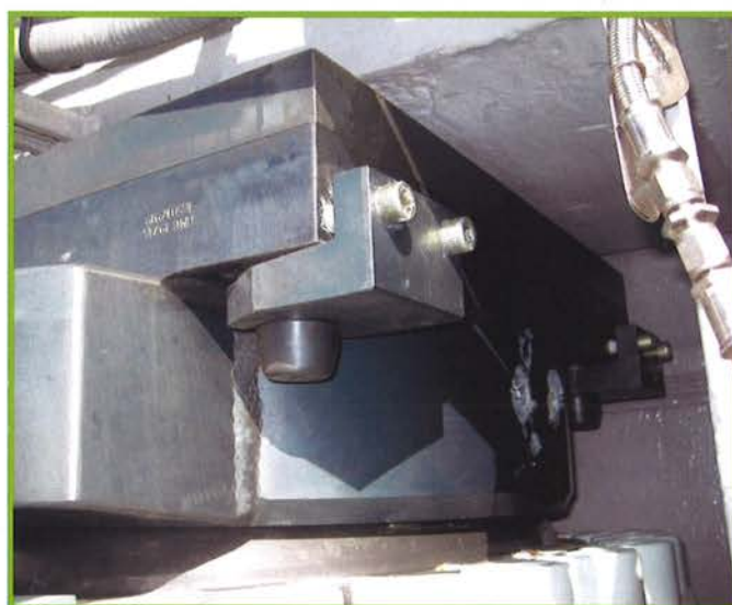
07 Mounting interface with fast locking wedges
