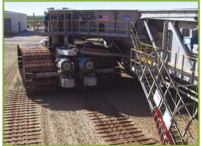
10 Cornering with the prototype JEL- cylinders at Kennedy Space Center
