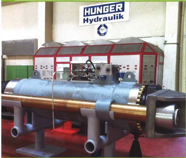
08 JEL- cylinder in the load frame on the hydraulic test rig
