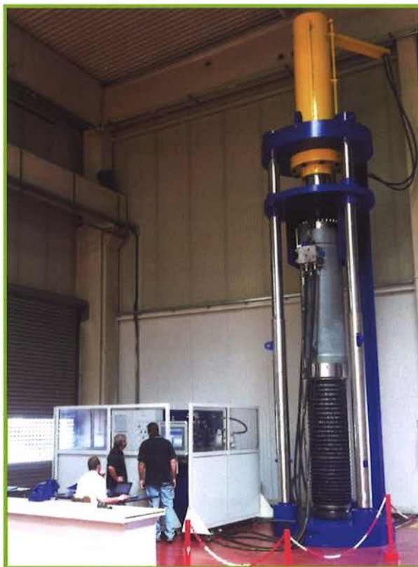
08 JEL- cylinder in the load frame on the hydraulic test rig
