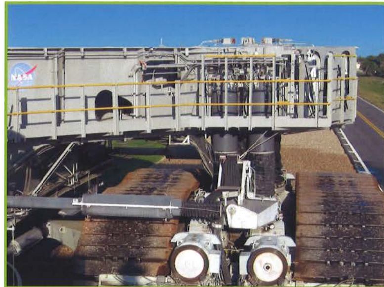
01 Installation situation of the old JEL- cylinders in one under-carriage
