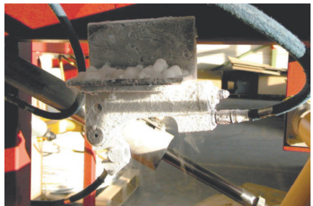
Locking hook for aviation technology at the low temperature of -54°C
