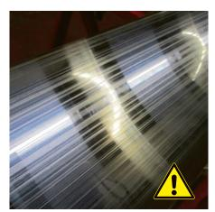
Machined seals and bearings are often made from semi-finished, extruded raw material bushings featuring material properties, which are strongly orientated in extrusion direction of bushing manufacturing process.
